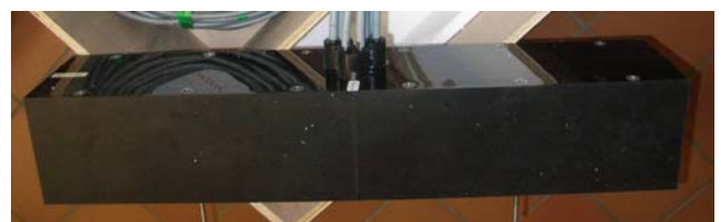
Fig. Reception Transducer of ATLAS HYDROSWEEP MD/50 (1° x 1.5°)
